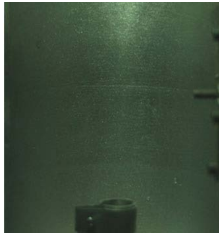
Figure 8. Image of thickness measurement of adherent liquid film under impinging angle 30°.
