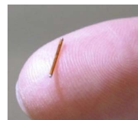
Figure 1. Shows the device concept that was utilized for stimulation. The nerve bundles were large, so a larger diameter device with and electrode surface area was constructed with the dimensions of 4.3 cm in length, 1.3mm in diameter, with a 0.6 mm diameter for the electrode spheres on each end. The original device was also evaluated, which is 1mm in diameter and 2 cm in length
