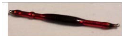
Figure 1. Shows the device concept that was utilized for stimulation. The nerve bundles were large, so a larger diameter device with and electrode surface area was constructed with the dimensions of 4.3 cm in length, 1.3mm in diameter, with a 0.6 mm diameter for the electrode spheres on each end. The original device was also evaluated, which is 1mm in diameter and 2 cm in length
