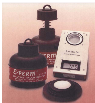
Figure 2. Radon Detection Kit, Showing Open and Close S-Chamber, Electret Disc Reader to the Right, and an Electret Disc Down Below.
