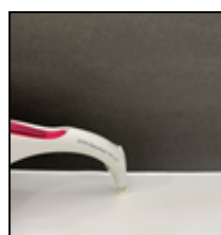
Figure 3. Spectrophotometer measuring the colour of the GIC samples before immersion.
