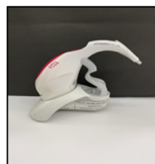
Figure 3. Spectrophotometer measuring the colour of the GIC samples before immersion.
