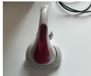
Figure 3. Vita EasyShade Spectrophotometer used for assessing the colour stability.
