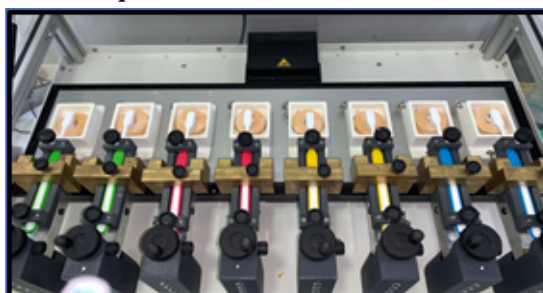
Figure 3. Shows the Brushing stimulator-Toothbrush stimulator ZM3.8 that was used for stimulating the brushing techniques on the restorative material.
