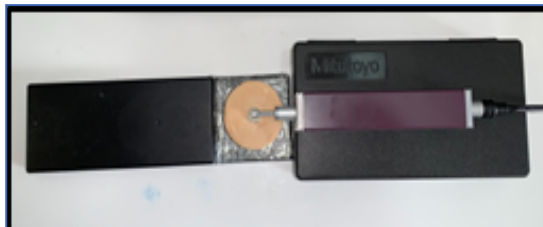
Figure 3. Shows the Brushing stimulator-Toothbrush stimulator ZM3.8 that was used for stimulating the brushing techniques on the restorative material.
