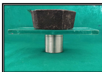
Figure 5. A weight of 1kg placed over glass slab for constant pressure.
