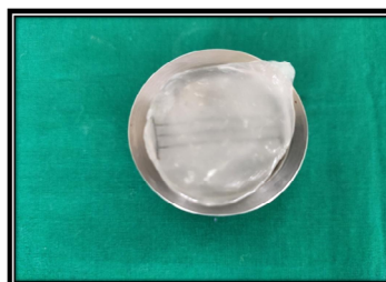
Figure 5. A weight of 1kg placed over glass slab for constant pressure.
