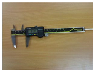
Figure 7- the digital vernier calliper having a measuring range of 0 - 15 cm with a range of 0.01 mm
