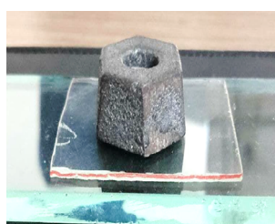
Figure 2 - Depicting the demonstration of the additional load of 100 gms kept over the initial glass plate measuring 20 grams . This gave a total load of 120 grams for the assessment of the flowability of the sealer.
