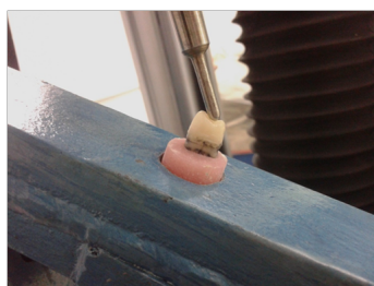
Figure 3. Position of the specimen in the setup for static loading (pressure forces was applied at an angle of 30 degrees on the inner inclines of support cusps).
